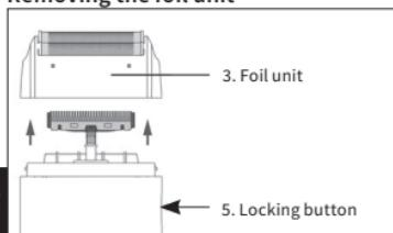
Press the locking button (5) on the side of the shaver; hold the foil unit (3) on both sides and gently pull it upwards.
