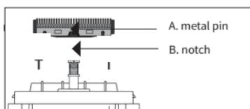
Remove the lamella blade: Hold it on both sides and pull it upwards.
